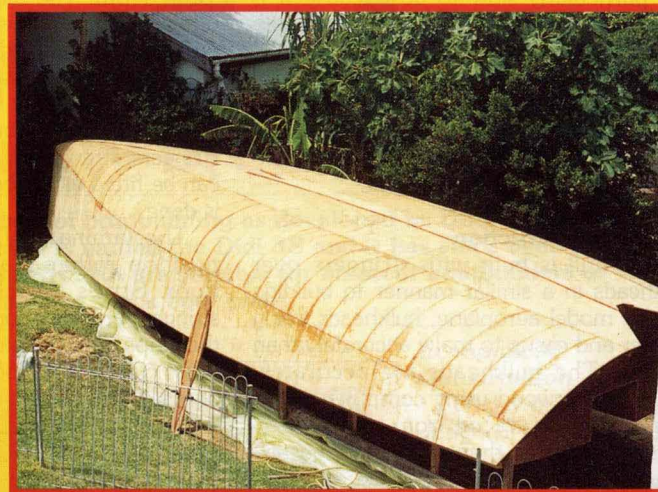
The skin is complete, and leaning against the hull is a hardwood shoe which will receive the keel.
