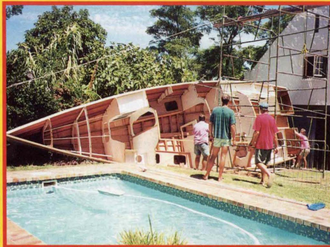
Turning her over before work commences on the interior and deck.
