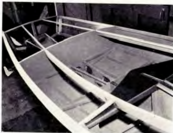
Part of hull before decking. This shows the double splayed webs forming the bifurcated keelson from aft of platebox to transom, in which are placed the flap valves for gravity-baling. These webs are covered within the after watertight compartment, forming a duct to the transom.
