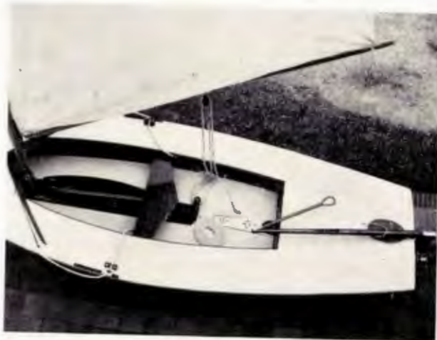
Plenty of room in this cockpit. It is 8 ft. long, the platebox is low and the wide reinforced plywood thwart makes a comfortable seat amidships.
