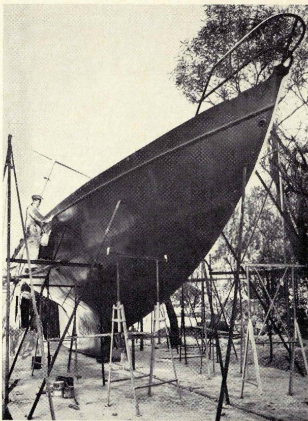
The first Alan Payne yacht to be built in the yard of E.S. Barends is shown on the left just as the plating was nearing its end and, on the right, the hydraulic press is "stretching" the subtle curve into one of the flat sheets.
